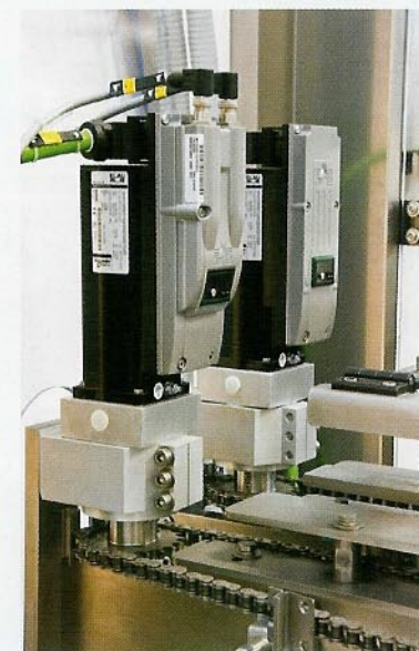
High-precision servo drives from ELAU help optimize performance on the Schuy overwrapper, used to wrap and stabilize the stacks of loaded trays.
