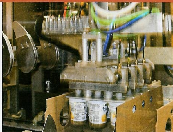
Vacuum-operated robotic suction grippers quickly place plastic containers into their exact spots inside the freshly-formed corrugated carrier trays.
