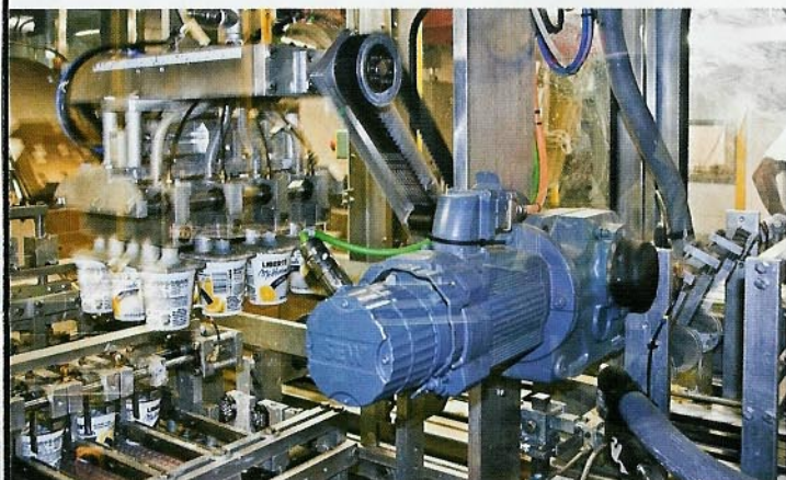
An SEW-Eurodrive motor controls power distribution for moving machinery and components inside the newly-installed case-packing station.
